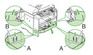
Push the paper cassette down until the hooks (A) on both sides of the paper cassette engage the protrusions (B) inside the machine.
